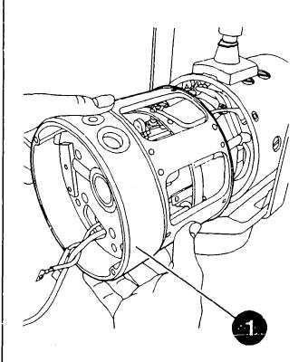
DISASSEMBLING DEEP-GROOVE BALL BEARING OF INTERMEDIATE BEARING
